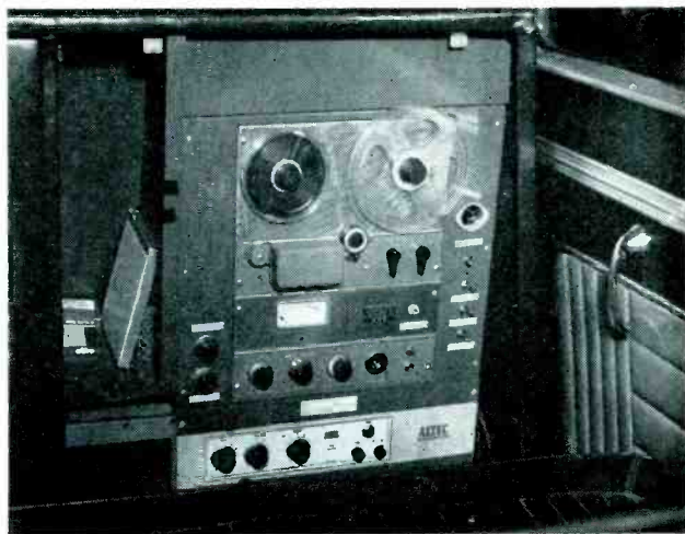
ABOVE: CUSTOM-BUILT car which features a complete public-address sound and 2-way radio system. At right is sound track tape recorder designed to be used to record voice announcements over the loudspeaker, phono records or radio. The recorder can be used while the car is in motion, and recordings played back directly through the loud speaker. While recording it is not necessary to have the material go through the loudspeaker. (Courtesy Miller Brewing Co.)
