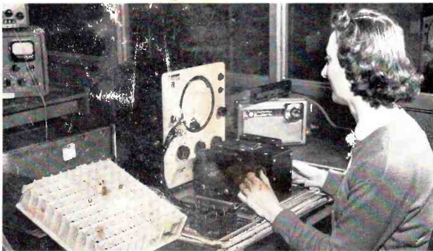
MODULE TESTING: Modular circuits are inserted on either side of bridge tester. One of the modules, a standard unit that has been previously deemed acceptable, is used as the standard in module tests. The tolerance or degree of variation between the two units shows up on the scale above the bridge. This test checks the resistance inductance and capacity deviation from the standard modular component.
