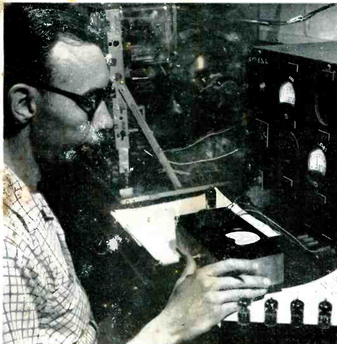
ELMER NIEHAUS testing video-amplifier tubes with special tube-checking setup. Equipment measures capabilities of video-amplifier pentodes to function without white-limiting or low gain.
