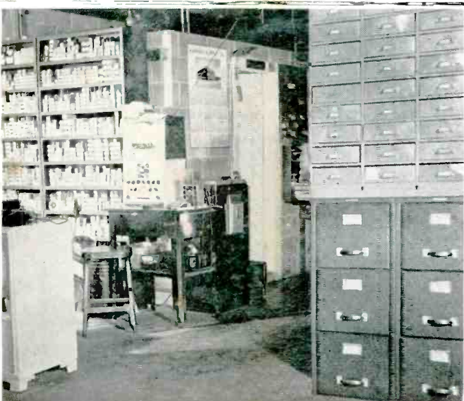
COUNTER-STOCK - record room in shop showing day-by-day service-call bulletin board and tube-test checking equipment on roll-about table.
