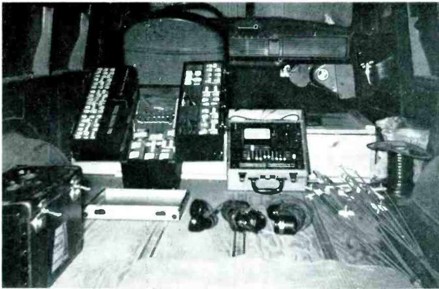
Interior view of truck used for TV and radio repair calls. Materials and instruments carried include tube caddy, tube checker, sound powered phones, antenna-installation kit, leadin and guy wire, antennas, roof and ladder hooks.
