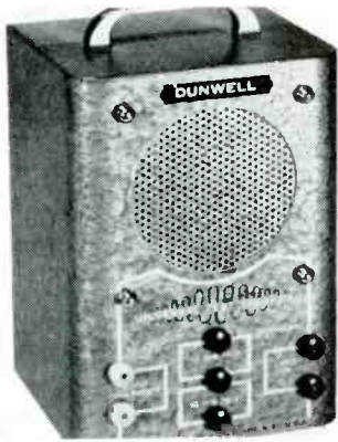
Test speaker designed for audio checks on TV, radio receiver or phono. Tip jacks connect to 4" pm speaker, universal output transformer, 60-ohm and 90-ohm fields. Test leads said to fit male or female speaker connections. (Universal test speaker, model A6 Dunwell Manufacturing Co., Carlstadt, N. J.)
