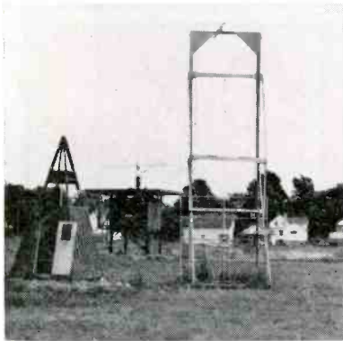
Fig. 2. Test site; antennas in foreground transmitting signal to receiving antennas on top of test house.
