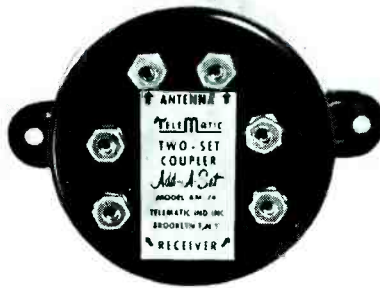
Add-a-set inductive coupler, utilizing a hi-core transformer, that operates two TV sets from one antenna on all vhf channels on either 72 or 300-ohm line. Unit is said to isolate antenna and receiver by the use of individual transformer windings, minimizing interreceiver action. (Model AM-74; Tele-Matic Industries, Inc., 1 Joralemon St., Brooklyn, New York.)
