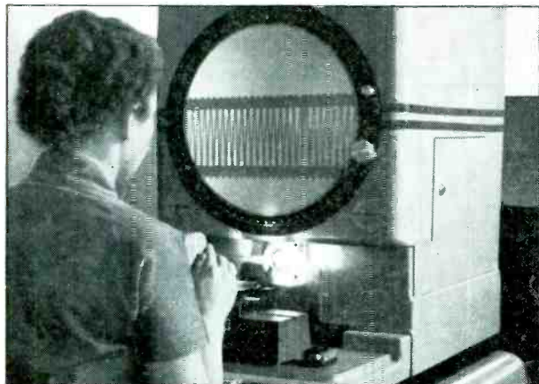
● A General Electric plant employee, using a comparator, checks a greatly magnified tube grid.
