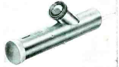
Wavemeter designed for uhf TV band. Covers a range from 400 to 1000 mc. Coupling to the wavemeter tuning element is said to be facilitated by use of an external coupling loop, so designed as to permit access to the portion of the circuit under examination. Absorption circuit consists of a high Q resonant cavity tuned by means of a slug-type split stator capacitor. (Model U-3; Linear Equipment Laboratories, Brightwater Place, Massapequa, L. I., N. Y.)
