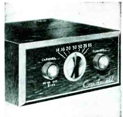
A uhf-TV converter, with a printed circuit tuner. Cabinet is 3 1/2" x 6 1/2" x 8" (Model ES-1; Allen D. Cardwell Mfg. Corp., 96 Whiting Street, Plainville, Conn.)
