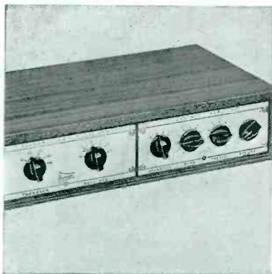
Audio control center, which consists of a phono preamp-equalizer, with separate turnover and roll-off controls, and control amplifier which provides input selector switch, bass boost and cut control, treble cutoff and boost control, and volume control. Features of the units are step switch controls for permanent calibration; universal pickup compensation; adjustable treble cutoff filter; maximum of 28 db bass boost; adjustable loudness control; low impedance output; tape recorder takeoff jack; and negative feedback. (Model A100-CA2; Brociner Electronics Lab., 344 E. 32 St., N. Y. 16.)
