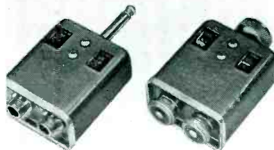
Miniature 2-input audio mixer, available with jack or mike connector inputs; accommodates two high impedance inputs. Connected directly to equipment—no external cables. Minimum lead lengths inside shielding housing said to minimize stray pickups. Separate gain controls for mixing. Gain control knobs recessed inside housing. (Model 310 with phone jack inputs—phone plug output fitting standard jacks, and model 320 with microphone connector inputs and output mating with standard microphone connectors; Switchcraft, Inc.)
