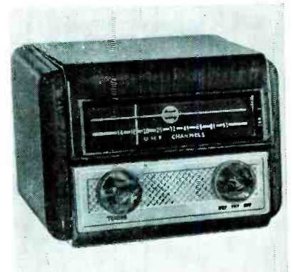
UHF-TV converter said to be especially designed for low-signal area installations. Features a two-section preselector with two silver-plated coax cavity tuners; double-shielded fundamental oscillator, and broadband amplifier with cascade circuit. According to the manufacturer, signal power loss in the preselector is reduced to 3 db; noise figure is a maximum 17 1/2 db to a minimum 15 1/2 db. Oscillator tube socket and all associated circuits are inside coax cavity, self-shielded to confine the normal oscillator signal. (TV-3; Turner Co.)
