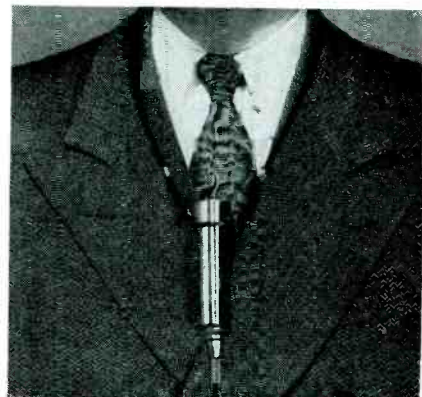
Six-ounce high-impedance microphone, with sealed crystal element, which is 4 1 / 2 " long and has a 1" diameter. Can be used on desk stand, as illustrated above, floor stand, or with lavalier, as shown below. (Slim-7 727; Shure Brothers.)
