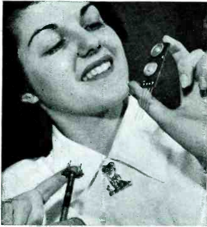
Comparing a printed-circuit if transformer and printed electronic circuit components. (Courtesy RCA)
