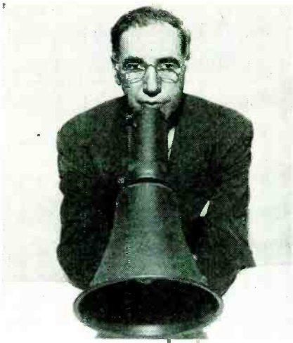
Megaphone using a transistor amplifier, demonstrated recently by Richard F. Shea, of General Electric's electronics laboratory. The amplifier units demonstrated achieved a peak power output of one watt.
