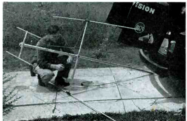
Fig. 2. While at the truck, and after antenna has been assembled, transmission line should be connected to the antenna.
