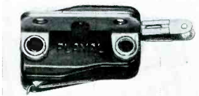
Dual speaker, designed primarily for railroad sound and other industrial installations, such as open pit mines, steel mills, factories, etc. Consists of a non-corrosive center aluminum casting with a weatherproof steel-bell reentrant speaker at each end of the opening. Velumoid gaskets between each cover plate and the casting are said to prevent any water seepage. Diaphragm is of bakelized linen. Magnet material is alnico 5. Voice coils are wound with aluminum wire. Diaphragm sensitivity is said to permit talk-back at distances up to 100'. Voice coil leads are beryllium copper gauze to relieve fatigue, and are welded. Dispersion angle per speaker is 45°. Frequency range, 350-6,000 cycles; total operating capacity, 40 watts; peak capacity, 70 watts. Impedance (speakers in parallel), 8 ohms. (Model RR-40; Racon Electric Co., Inc., 52 East 19th St., New York 3, N. Y.)
