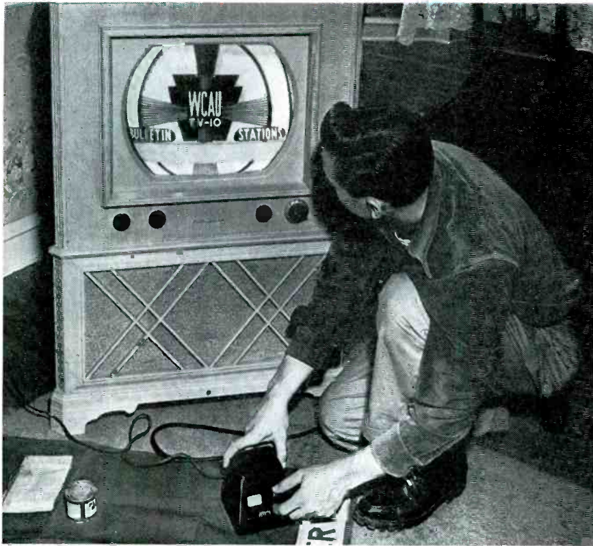
Fig. 1. Orienting the antenna with a rotator.
