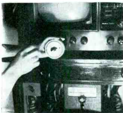
Fig. 6. Adjusting tunable stub to eliminate if interference in the 26 to 32-mc band.
