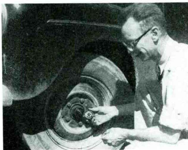
Installing noise suppression grounding springs in front wheels.
