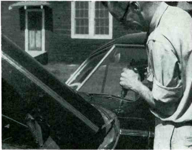
Cutting antenna mounting hole with circle cutter.
