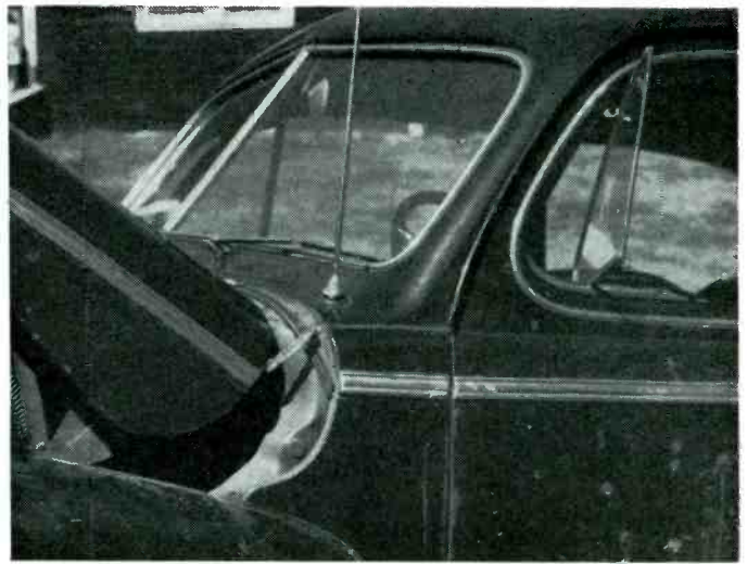
Top-cowl mounted antenna. Note flexible strap bonding hood to body just below antenna, also hood grounding spring just below hood.
