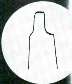
Horizontal sync-pulse as displayed on WO-57A screen
