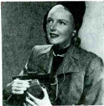
Figs. 6 (above) and 7 (below). In Fig. 6 appears a Belmont pocket receiver using the new sub-miniature type tubes. Receiver is 3 " wide, 3/4 " thick, and 6\frac{1}{4} " high. Weighs about 10 ounces, including batteries. Fig. 7 shows a cross-sectional view of the sub-miniature tube used in the receiver.
