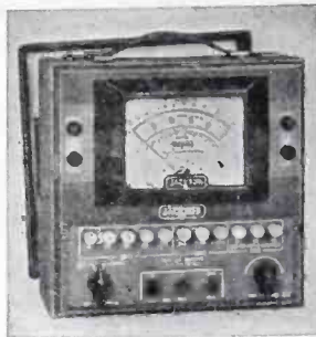
Sensitive Multimeter Model 642—20,000 ohms per volt—complete ranges
