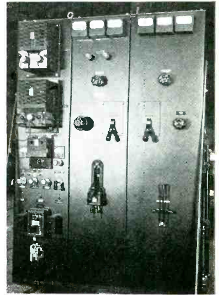
Figs. 4 (left) and 4a (above). In Fig. 4 we have a three-phase full-wave circuit with six thyratrons. Fig. 4a shows an a-c voltage indicator unit used in electronic voltage regulation systems.
