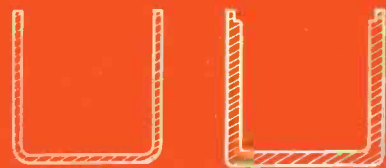
DRAWN ALUMINUM TO BAKELITE SAVING 100% ALUMINUM
