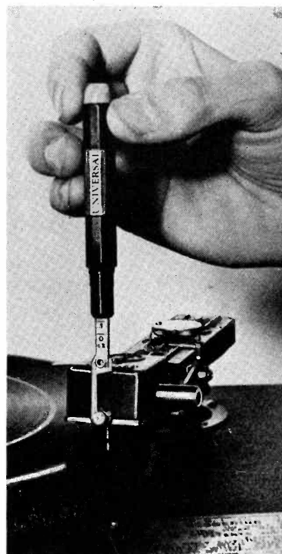
Fig. 3. A small weight scale for determining the pressure exerted by a phono pickup or recorder head on the needle. A hook is provided for lifting.
