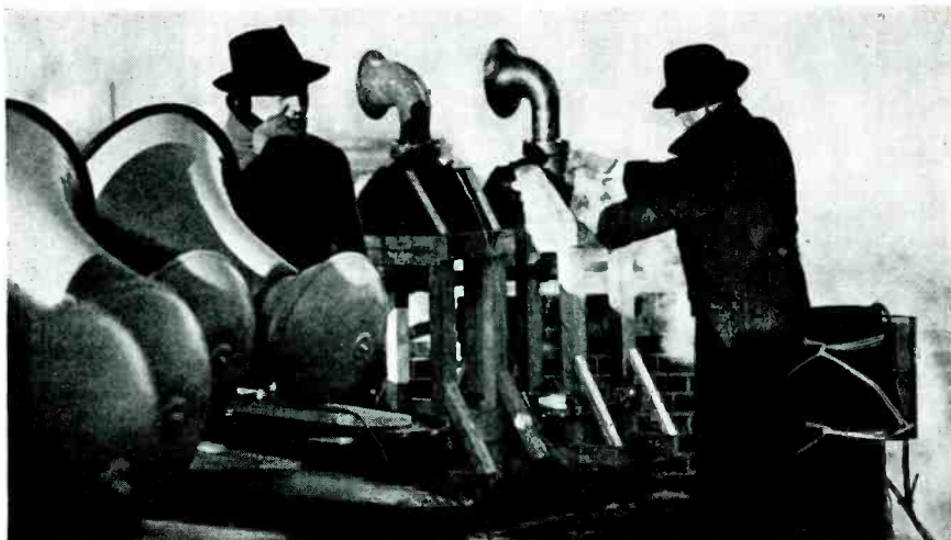
Fig. 3. Sound systems have several distinct advantages over other equipment when used to give air raid alarm signals. The trumpets shown above were used in a test in Newark, N. J.
