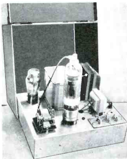
Fig. 1. Automatic control unit through which applications of welding current are limited to single impulses of less than 1/120 second. The tube in the foreground is the type C6J discussed in the text.
