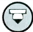
Shaft position in knob requiring 1/32" flat.
