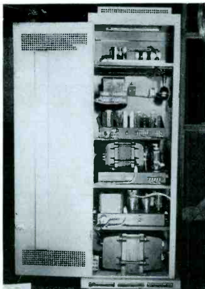
Fig. 2. A 500-watt amplifier supplies power to drive a motor at absolutely constant speed for Curtiss-Wright.
