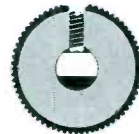
How shaft is positioned for set-screw knob.
