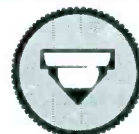
Shaft position in knob requiring 3/32" flat.
