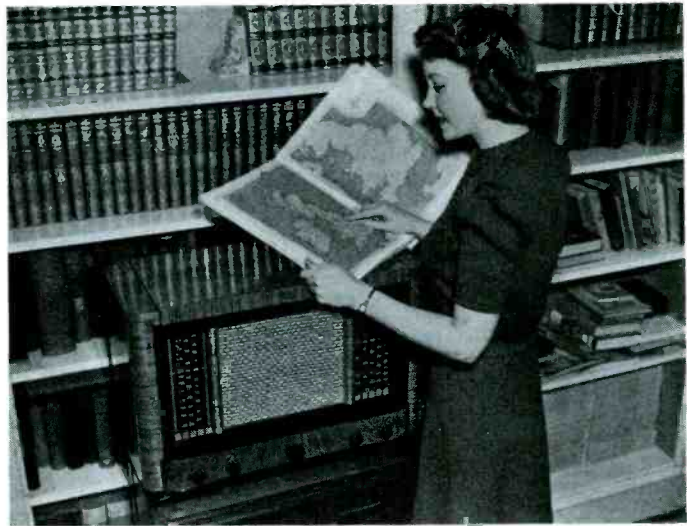
Fig. 1. A trend toward the use of dual vertical dials, as shown in the Philco 41-788T to the right, is evidenced in the 1941 models. On all-wave sets the extra dial is used for band spread tuning; on f-m combinations one dial is used for a-m and the other for f-m.
