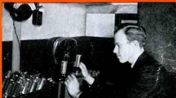
Every Mallory Vibrator is tested for noise in a sound-proof room under actual set operating conditions.
