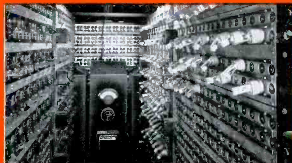
Life test. A percentage of every production run on every type of Mallory Vibrator is tested under actual set operating conditions for 1000 hours.
