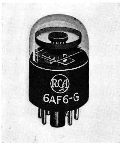
RCA 6AF6-G visual indicator tube, a typical dual indicator type.
