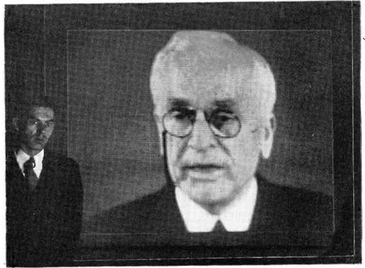
A photograph of the 4 x 5 foot projected image reproduced by Kolorama Laboratories television apparatus.
