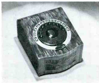
Fig. 1. The Philco Mystery Control unit. The battery operated oscillator and pulser mechanism, shown on the front cover, are located in this box.
