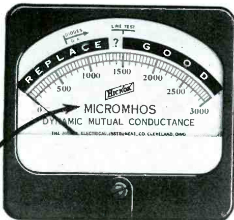
Meter used in HICKOK T-53 TUBE TESTERS. RANGE: 0-3000-6000-15,000 MICROMHOS.
