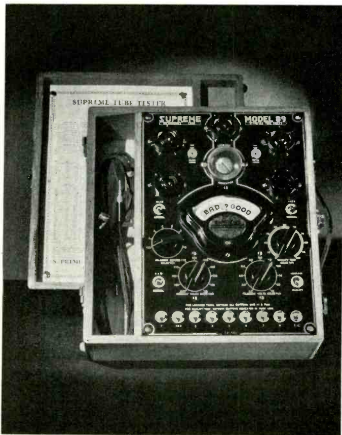
The new tester for the 8-pin tubes, incorporating the "filament return selector."
