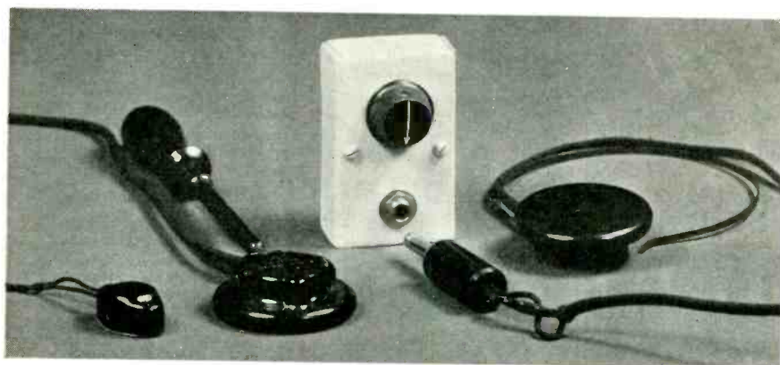
Fig. 2. Showing a typical outlet box, with jack and volume control, and two types of light-weight phones. A bone-conduction unit is shown at the extreme left.
