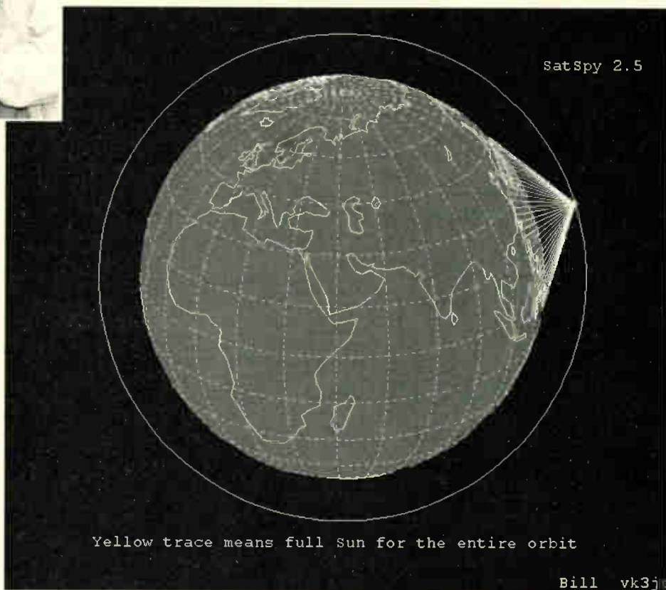
Graphic showing the KITSAT-OSCAR-23 satellite in constant sunlight late last year. The lack of eclipses causes a dramatic temperature rise on the spacecraft, thereby resulting in a distorted downlink signal and sharply reduced throughput.
