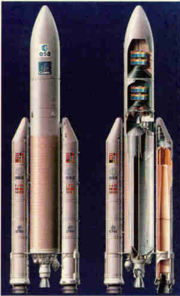
Outside and cut-open view of the Ariane-5 launcher configured for its maiden flight with a payload of four identical CLUSTER satellites. The first launch was a failure.
