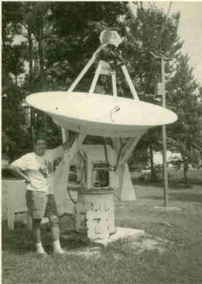
Dr. Dave Moore with military surplus antenna, redesigned for radio astronomy use.
