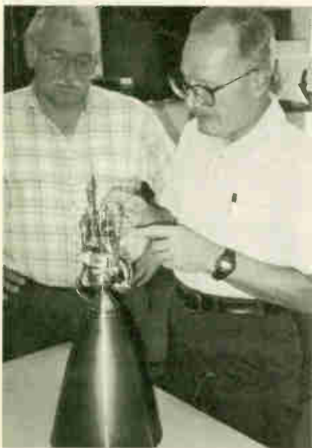
AMSAT-NA Vice President, Engineering Dick Jansson, WD4FAB (Right), and AMSAT-DL's Konrad Mueller, DG7FDQ (Left), perform a final inspection of Phase 3-D's 400 Newton kick motor in Konrad's well-equipped machine shop at AMSAT-DL prior to its shipment to Orlando for integration. The motor is of the same design that successfully powered both AO-10 and AO-13 to their final orbits.
