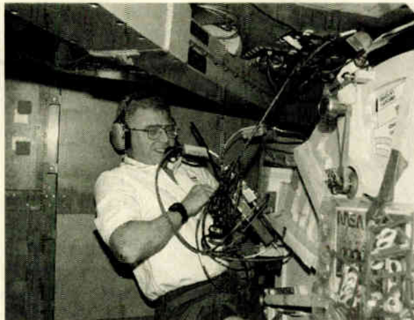
Among the Inflight Maintenance (IFM) chores that were handled by the crew members during their almost 17 days in space aboard the space shuttle Columbia was one that involved going into the bay beneath the floor of the Life and Microgravity Spacelab (LMS-1) Science Module. Astronaut Terence T. (Tom) Henricks, mission commander, shines a tiny flashlight onto some cables related to LMS-1 supported computer systems. As in the case of the other IFM chores, Henricks efforts were successful. He was joined by four other NASA astronauts and two international payload specialists for the space shuttle duration record-setting mission. (NASA)
