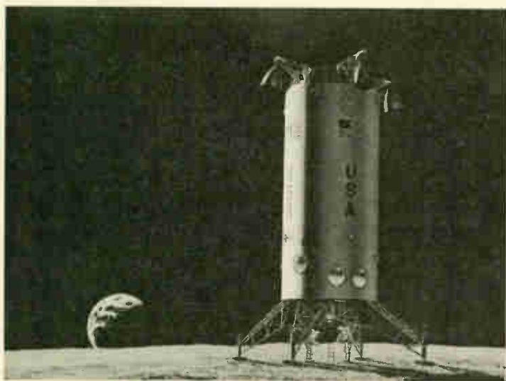
An artist's concept for a cylindrical lunar lander showing round windows, main thrusters at the top of the vehicle and maneuvering thrusters around the circumference of the vehicle. (Lockheed Martin Missiles)
