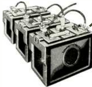
Three heavy duty rubber jar 6-volt radio batteries connected in parallel, thereby tripling storage capacity but remaining at 6 volts.
