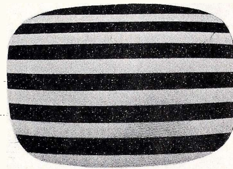
Fig. 4. 400-cycle modulation with poor vertical linearity.
