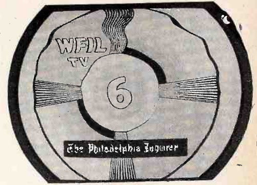
Fig. 7. Hunting by control tube produces this effect.
