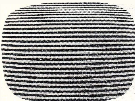
Fig. 5. 1500-cycle modulation with poor vertical linearity.
