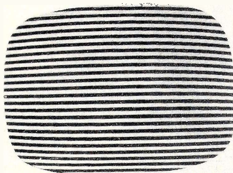
Fig. 3. Pattern produced by signal generator with 1500-cycle modulation.
