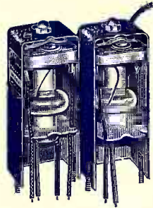
Inside view of I.F. transformers. The output type usually has four leads at the bottom. The input and interstage types have the grid lead coming out of the top.
