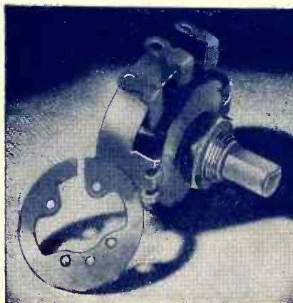
Potentiometers are used as volume and tone controls. Usually there are three terminals, but a fourth tap may be found on some special units.
