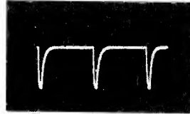
V201B PIN 1 SYNC PLATE HORIZONTAL RATE 60V P-P
