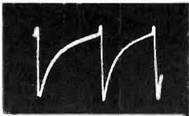
V206B PIN 9 VERTICAL OSCILLATOR GRID VERTICAL RATE 180V P-P
