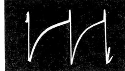
5 V206B PIN 9 VERTICAL OSCILLATOR GRID VERTICAL RATE 140V P-P
