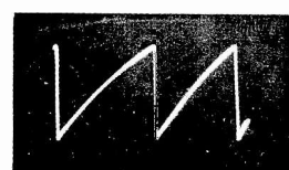
⑥ V206A PIN 2 VERTICAL OUTPUT GRID VERTICAL RATE 28V P-P
