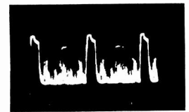
14 R224 & C246 JUNCTION ZONE 7A PW200 BOARD HORIZONTAL RATE 90V P-P
