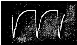
② V101 PINS 2 & 6 HORIZONTAL OUTPUT GRID HORIZONTAL RATE 130V P-P
