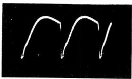
12 SR201 CATHODE JUNCTION HORIZONTAL PHASE DETECTOR HORIZONTAL RATE 12V P-P
