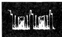
⑧ V205B PIN 9 VIDEO AMPLIFIER PLATE HORIZONTAL RATE 110V P-P
