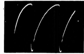
Horizontal oscillator plate, pin 6 of 12AU7A (S4E), 165 volts, 15,750 c.p.s.
