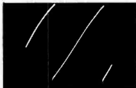
Vertical oscillator plate, pin 6 of 12AU7A (S3E), 110 volts, 60 c.p.s.
