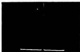
Vertical oscillator cathode, pins 3 and 8 of 12AU7A (S3E), 23 volts, 60 c.p.s.
