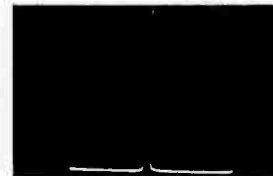
Vertical oscillator plate, pin 1 of 12AU7A (S3E), 120 volts, 60 c.p.s.
