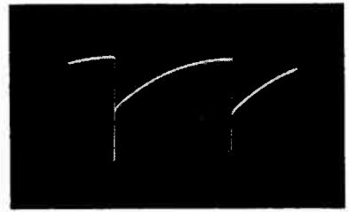
Fig. 14. Vertical-Output Grid, Pin 2, 72 volts, 60 c.p.s.
