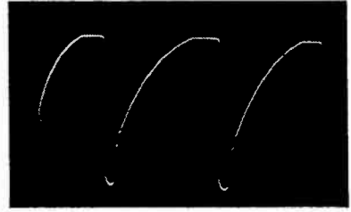
Fig. 20. Horizontal-Output Grid, Pin 5, 120 volts, 15,750 c.p.s.
