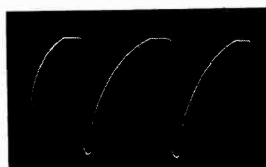
Fig. 20. Horizontal-Output Grid, Pin 5, 160 volts, 15,750 c.p.s.
