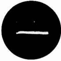
← Plate of sync clipper (pin 5 of V-17, 6SN7), 30 volts peak-to-peak — 60 cps.
