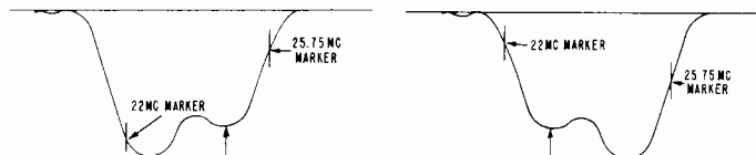
Figure 6. IF Response Curves, Incorrect Shape.
