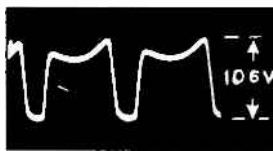
Pin 6 12AX7 (V9A) 60 cycles
