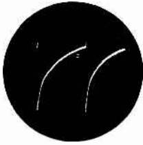
← Yellow lead to T-11, 50 volts peak-to-peak — 60 cps.
