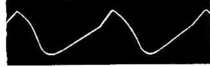
No. 18—6W4 Damper Plate 120V P-P 15,750 C.P.S.
