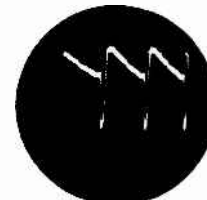
←←← Cathode of phase detector (pin 5 of V-25, 6AL5), 13 volts peak-to-peak — 15.75 Kc.
