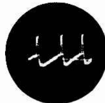
←←← Plate of phase detector (pin 7 of V-25, 6AL5), 12 volts peak-to-peak — 15.75 Kc.
