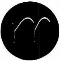
← Red lead of vertical output transformer T-10, 70 volts peak-to-peak — 60 cps.
