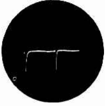
← Output of vertical integrating network M-1, 25 volts peak-to-peak — 60 cps.
