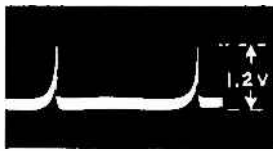
Pin 1 12AX7 (V9B) with red & bl of T6 shorted 60 cycles
