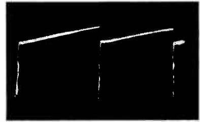
Fig. 14. Vertical-Output Grid, Pin 6, 80 volts, 60 c.p.s.
