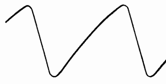
Figure 16. Waveform on Grid Pin 1 of V403 Without Sync Pulse.
