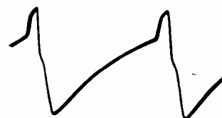
Figure 15. Waveform on Grid Pin 1 of V403 With Sync Pulse.
