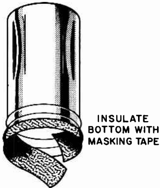
Figure 29. Tube Shield for IF Alignment and IF Response Curve Check.
