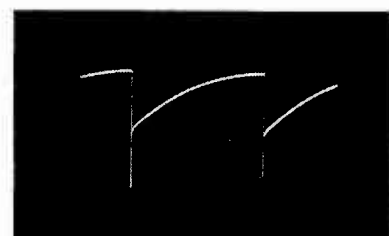
Fig. 14. Vertical-Output Grid, Pin 2, 72 volts, 60 c.p.s.
