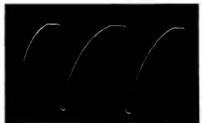
Fig. 20. Horizontal-Output Grid, Pin 5, 160 volts, 15,750 c.p.s.
