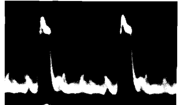
FIG. 5-29 HORIZONTAL PULSE 9 Volts PP
