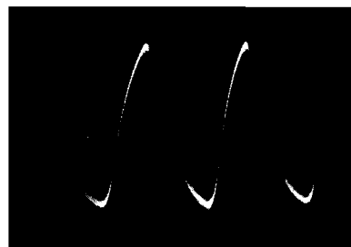
Fig. 86. Pin No. 5 V209 (Horizontal) P-P—6V.
