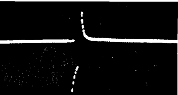
FIG. 5-42 VERTICAL PULSE 1.6 Volts PP
