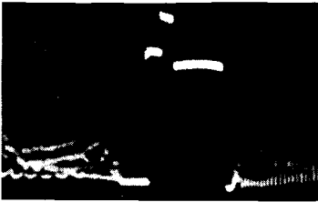
FIG. 5-28 VERTICAL PULSE 9 Volts PP
