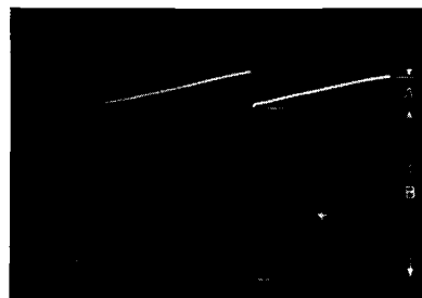
Figure 64 Pin No. 2 V220B (Plate vertical saw generator) A—10V B—110V
