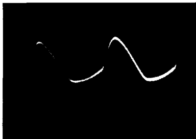
Figure 79 Same point as Fig. 78. Signal observed when not tuned to a channel. 5V—p-p.
