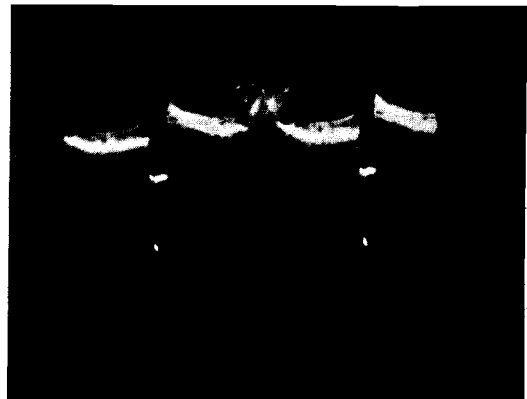
Figure 5. Video Signal at Pin #7 (plate) of V204
