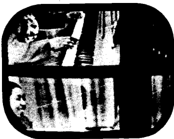
Fig. 88. Picture out of sync both horizontally and vertically.
