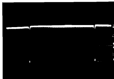
Figure 58 Pin No. 4 V220A. (Grid 6SN7 vertical buffer) A—19V B—19V
