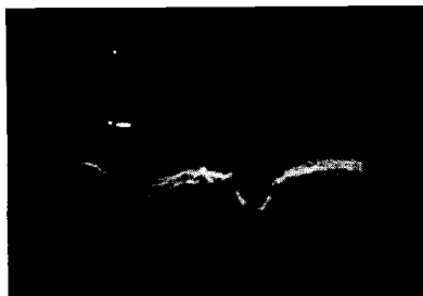
Figure 54 Pin No. 1 217 (Grid sync clipper 6AG5) (Vertical) 12V p-p.
