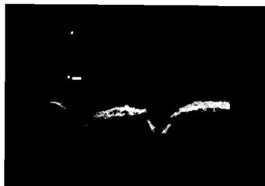
Figure 52 Junction of L215-R223 plate circuit of V205, 1st video amplifier (Vertical) 16V p-p.
