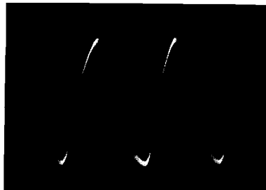
Fig. 85. Pin No. 7 V209 (Horizontal) P-P—6V.
