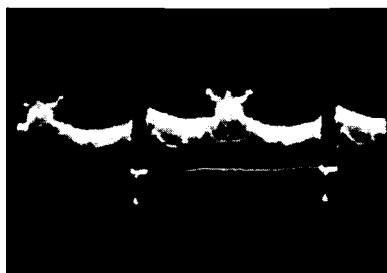
Figure 50 Pin No. 3 V207 (Plate 3rd video amp. 6K6) 47V p-p.
