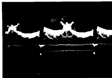
Figure 40 Pin No. 7 V204 (Video detector plate) (Field) 1.4V p-p.
