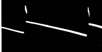
FIG. 5-43 HORIZONTAL PULSE 1.0 Volts PP
