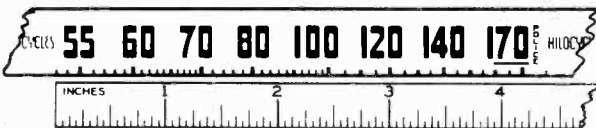
Receiver Dial Scale and Corresponding Calibration Scale
