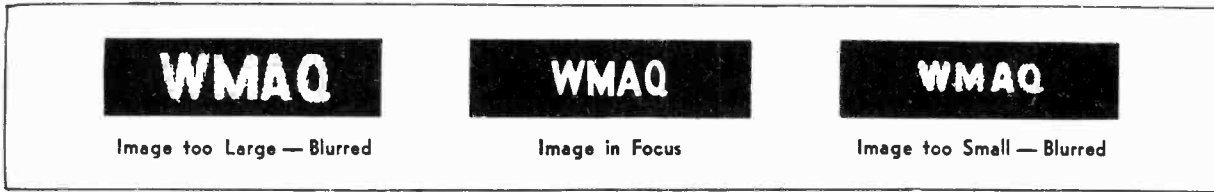
Fig. 7—Effect of Lens Focus
