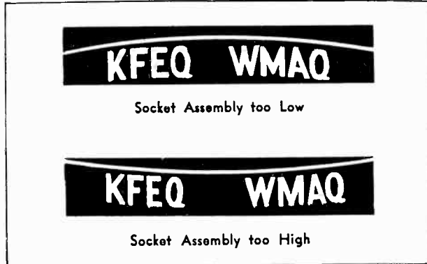
Fig. 5—Effect of Lamp Socket Assembly Height
