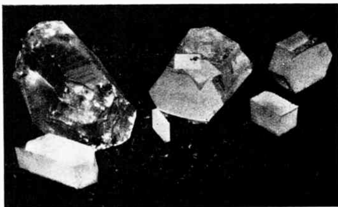
A piece of raw quartz and several unfinished slabs from which oscillating crystal blanks are cut. The best quartz is mined in Brazil.
