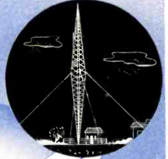
1930 Half-wave vertical radiator, now in general use, was developed into practical form. It greatly improved signal output of broadcast stations.
