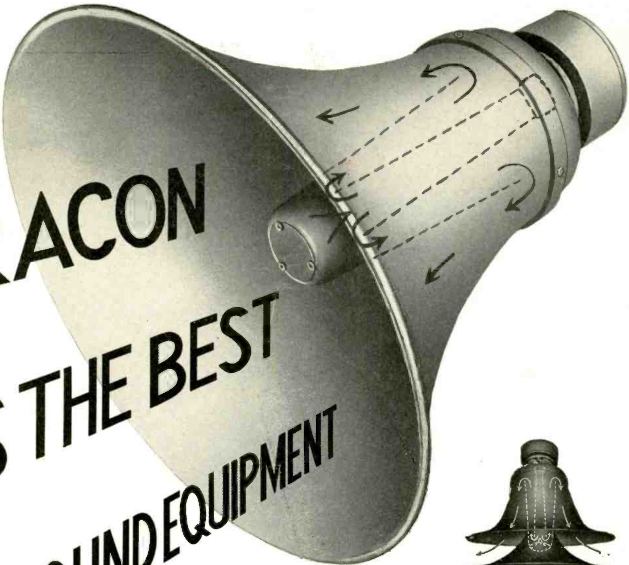
RADIAL HORN SPEAKER; a 3 1/2' re-entrant type horn. Projects sound over 360° area. Storm-proof. Made of RACON Acoustic Material to prevent resonant effects.
