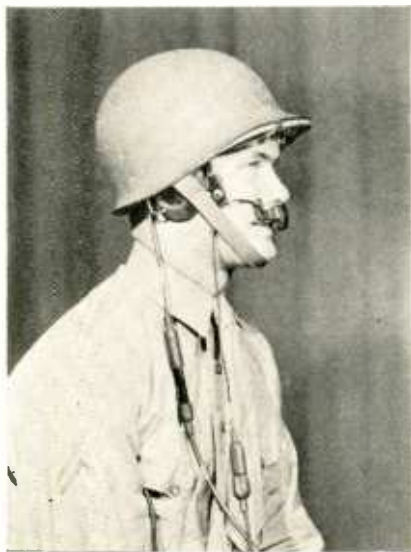
This new "submersion-proof" Western Electric lip microphone and headset combination was developed by Bell Laboratories. The microphone is fitted with a gland which will pass air but exclude water
