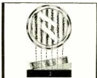
Optical Flat. Surface of Work. Interpretation of bands on truly flat surfaces.
