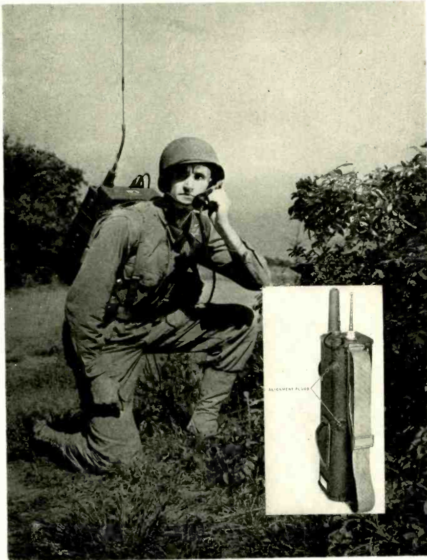
Signal Corps FM walkie-talkie being operated by soldier in training. Inset shows Handi-Talkie radio SCR-536 — Signal Corps Photo
