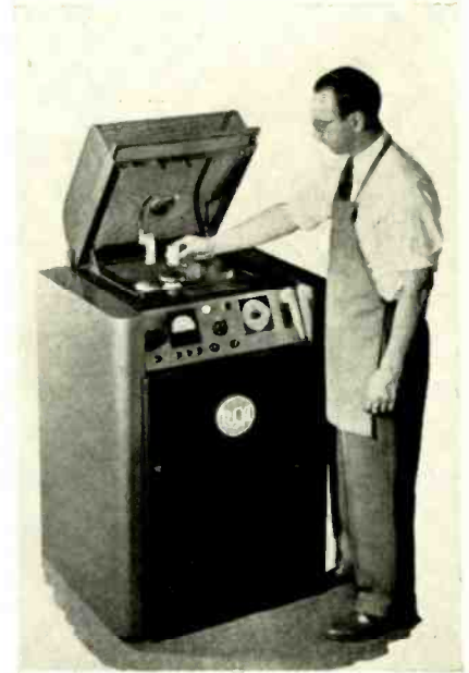
New RCA electronic pre-heater for plastics. At the end of a pre-determined heating interval, the lid automatically pops up
