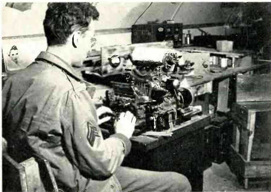
Signal Corps repair depot in Iceland. Shown is repairman testing a Teletype machine after general overhauling. In background is a Hallicrafters SX-25 receiver used for the reception of vital information at the depot. (U.S. Army Signal Corps photo.)
