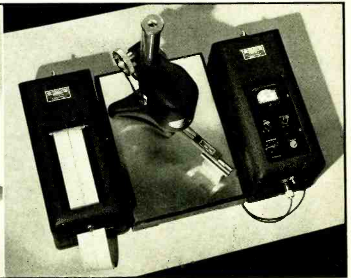
Fig. 11. A complete surface analyzer consisting of a direct inking oscillograph, drive head on surface plate, and a calibrating amplifier.
