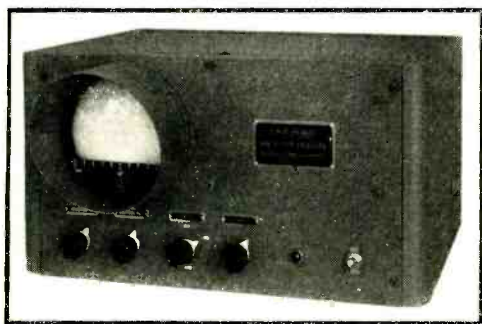
Figure 2A. Front view of a commercially manufactured version of the panoramic radio spectro-scope.
