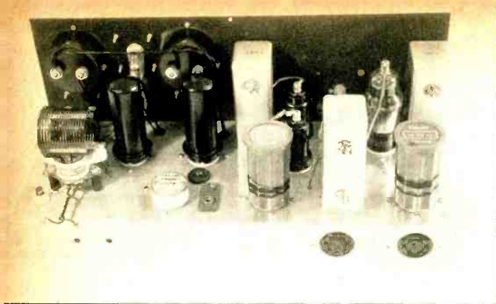
Rear view of the transmitter-receiver deck of the portable station. The two-tube r.f. section of the transmitter is mounted to the left of the center of the chassis; the receiver portion is mounted to the right of the chassis center line.
