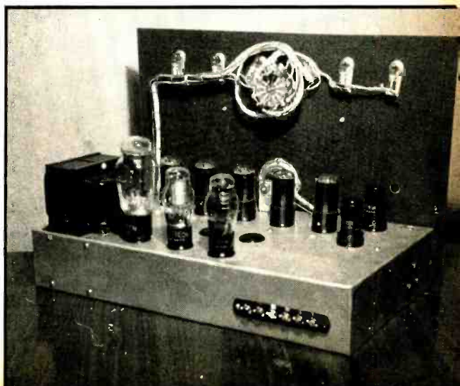
Rear view of the exciter chassis. Note that the power supply is on the extreme rear.
