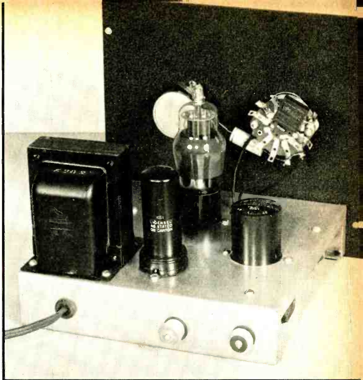
Figure 1. Illustrating construction of the universal phono equalizer and scratch reducer.
