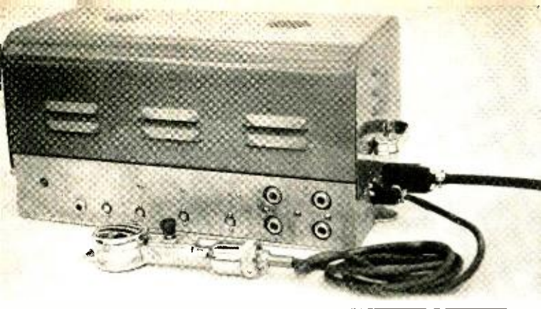
The complete transmitter unit, with the dust cover in place, makes a very neat installation. Note that the mike is in the remote control jack for making an adjustment on the transmitter.
