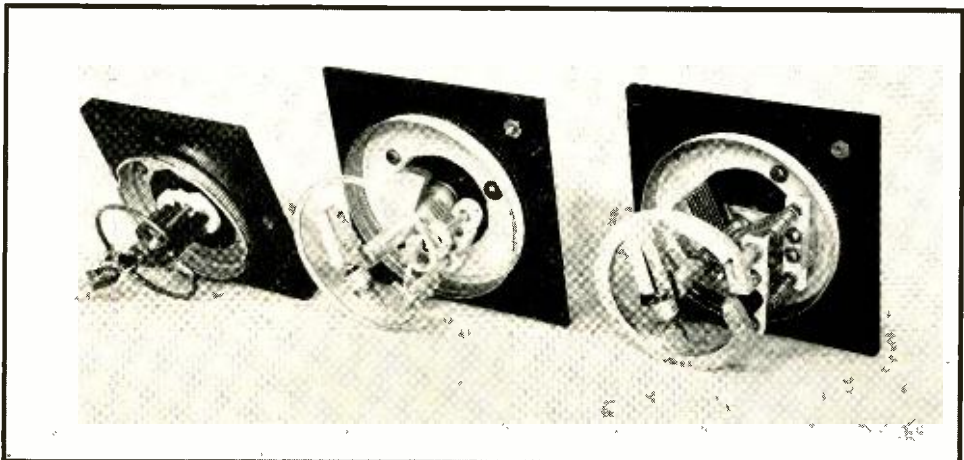
Figure 1. The three u.h.f. wavemeters. From left to right they are: no. 1, the one using the APC-75 condenser; no. 2, with an MC-50-M in the center; no. 3, with the 270° straight-line frequency condenser, is on the right.
