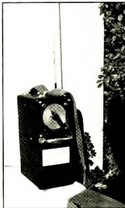
The pack set of W6EL, used for taking accurate bearings simply by making use of one's body as a reflector.
